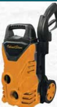
Voltage 230-240V/50HZ. Maximum pressure 105 BAR. Flow rate 5,0L/min. Pump with axial piston oscillating. Pistons in stainless steel tempered. Automatic suction function to load water directly from a bucket or drum. Two-wheeled trolley and handle for easy movement. Start/stop automatic function. 5M electrical cable. 3M high-pressure tube. Lance with adjustable nozzle and lock. Power 1400W
