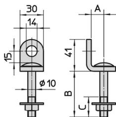
OCCHIOLI FISSI - INDICATI PER: LUCCHETTI CORAZZATI FAI BY VIRO, PANZER, PANZER INOX, PANZER PREDISPOSTI PER MEZZO CILINDRO E MONOLITH
